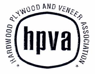
FLAME SPREAD 200 OR LESS CLASS C ASTM E 84
